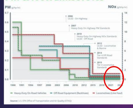
New Technology Diesel Engines for commercial trucks, farm tractors, construction machines, generators sets, rail, all now achieve near zero emissions, are more fuel efficient and lower in GHG emissions; all are capable of using low-carbon biobased diesel fuels.
