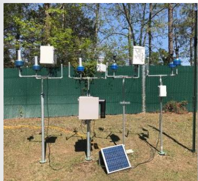
Fence-line monitoring devices (SPods)
