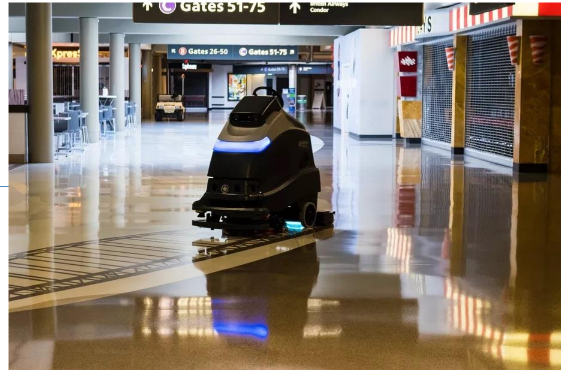
A UV scrubber at Pittsburgh International Airport. Photo: Pittsburgh International Airport
